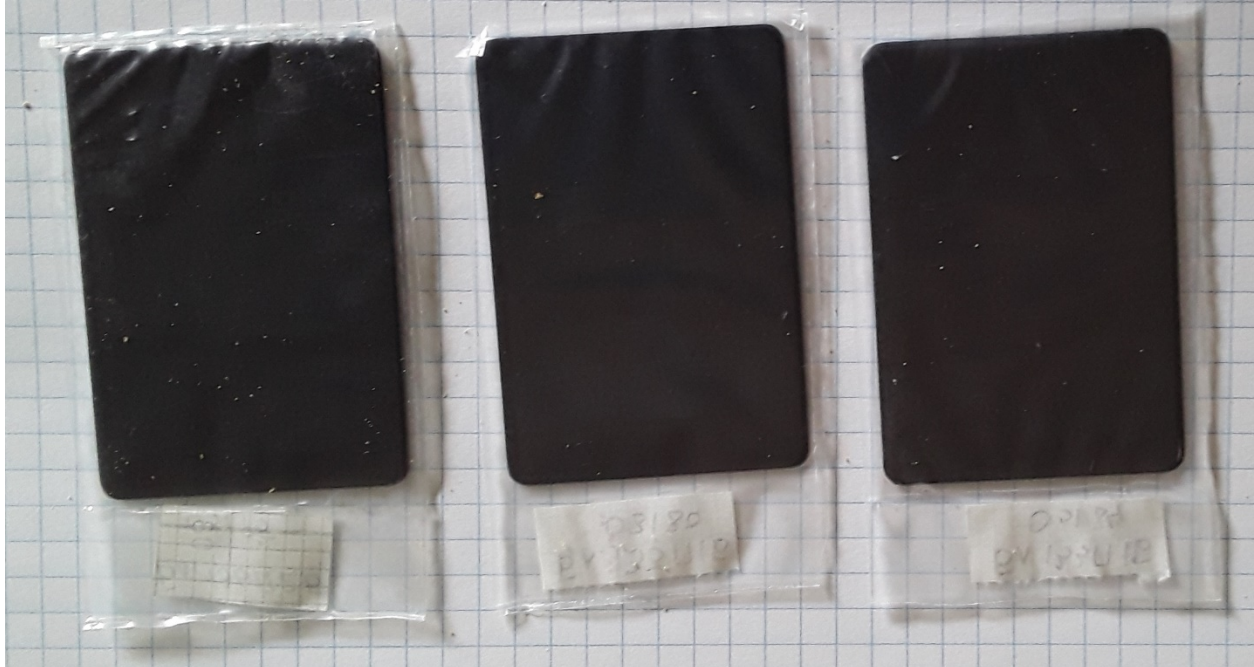
Fig. 17. Examples of MCP with dimensions 60x40 mm.
