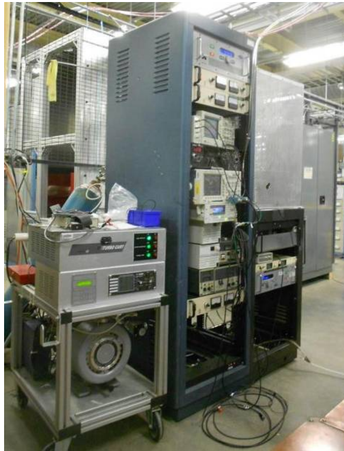
Fig. 21. A test stand for electron beam testing (front left side) was designed, fabricated, assembled, and prepared for work. The Manual and Safety & Hazard instructions were prepared, reviewed, and approved. The test stand was commissioned, and electron beam testing followed.
